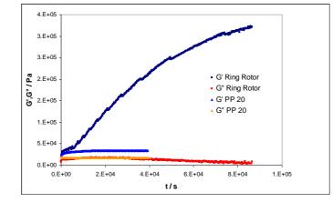
Figure 1: Storage modulus G' and loss modulus G" versus time for a polyurethane sealant, determined with a) 20 mm plate-plate geometry and b) newly designed ring rotor at ambient conditions, f = 1 Hz,  $\gamma = 1$  %.
